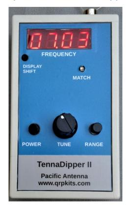
The "Tenna Dipper" provides a simple means of determining the 50 ohm resonant frequency of an HF antenna or ATU (Antenna Tuning Unit).
