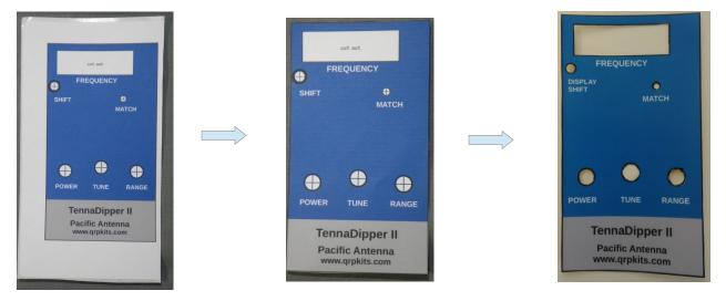
If not, leave these and you can use the case holes as a guide to trim the holes using an Exacto knife once it is applied to the panel.
